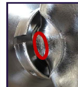
Burst happened at the connection of stiffening ring to half cell
