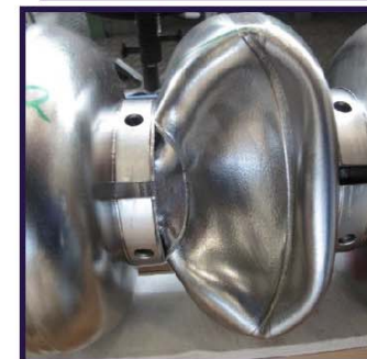
Burst happened at the connection of stiffening ring to half cell
