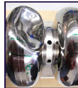
LG cavity after burst test. How painful for us was to look on this.
