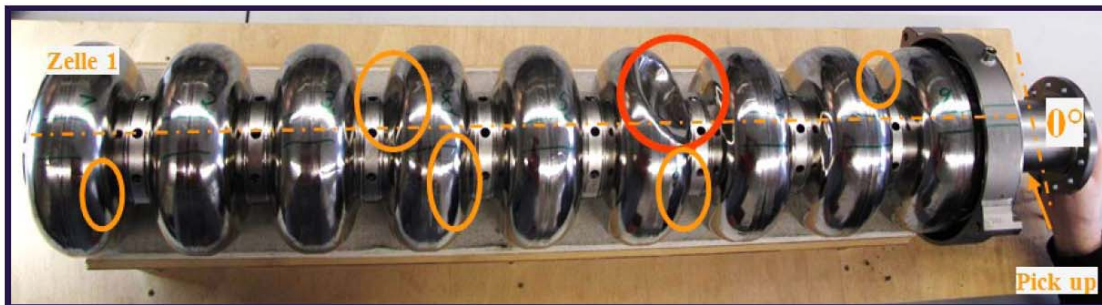
LG cavity after burst test. How painful for us was to look on this.
