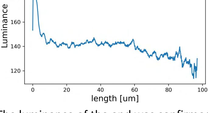
The luminance of the end was confirmed. The dE/dx should be bigger for Alpha recoil tracks.
