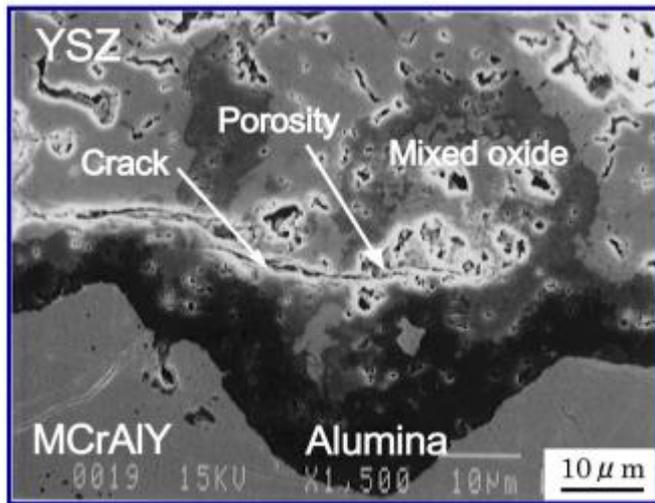
Cross-sectional SEM image of TBC aged for 3000 hours at 1000°C
