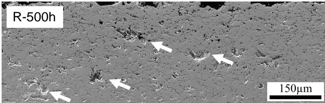
Cross-section morphology of top coat in a large range
