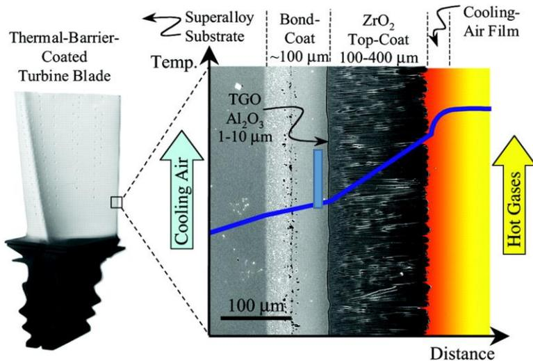
Photograph of a turbine blade with thermal barrier coating (TBC)
