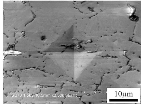
no obvious cracks are caused by the indentation test
