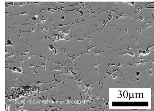
1. healing of micro-cracks and micro-pores due to sintering effects
