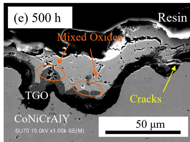
Topcoat separation occurred after heat treatment at 1100°C for 500 h in air.
