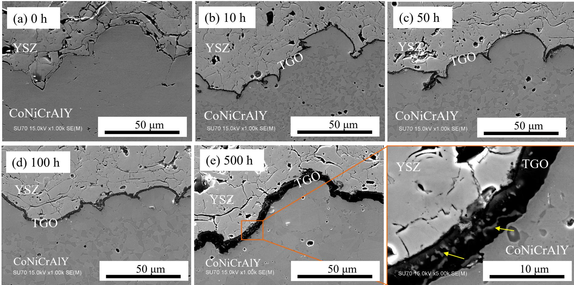
No separation occurred at TC-TGO interface after heat treatment at 1100 °C in 5% H<sub>2</sub> for 500 h.
