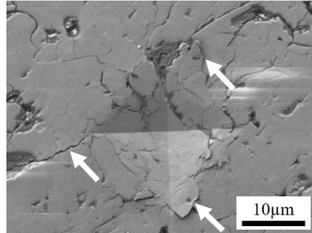
Cracks generate and propagate at the location of pre-existing microcracks.
