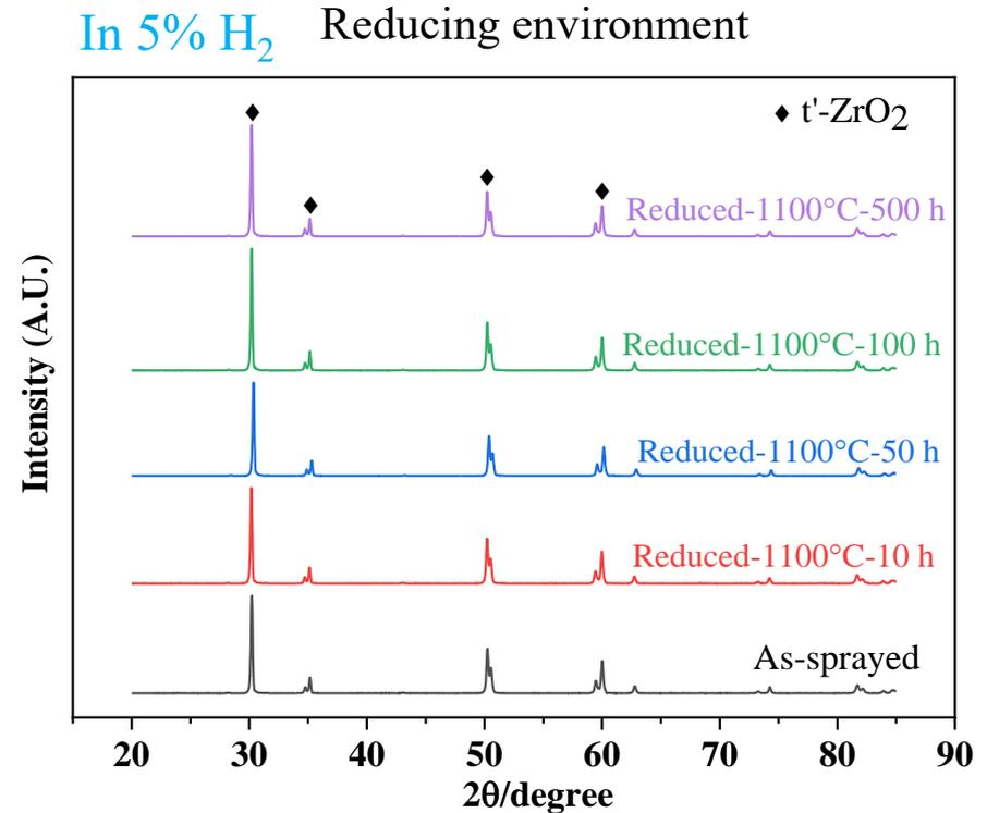
XRD results show that after heat treatment at 1100°C for 0~500 h, the topcoat surface of TBCs samples consist of t'-ZrO<sub>2</sub>, which means there is no any phase transformation of the topcoat surface under **both** environments.
