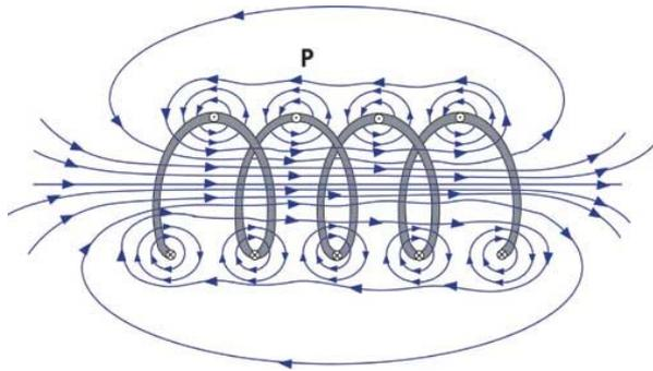
$$e(t) = - \iint_{coil\_surface} \frac{\partial \vec{B}}{\partial t} \cdot \vec{dS} = -L \frac{di(t)}{dt}$$
