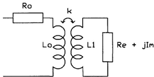
$$Z_0 = R_0 + jX_0 \quad R_{CN} = \frac{R_C - R_0}{X_0} \quad X_{CN} = \frac{X_C}{X_0}$$
