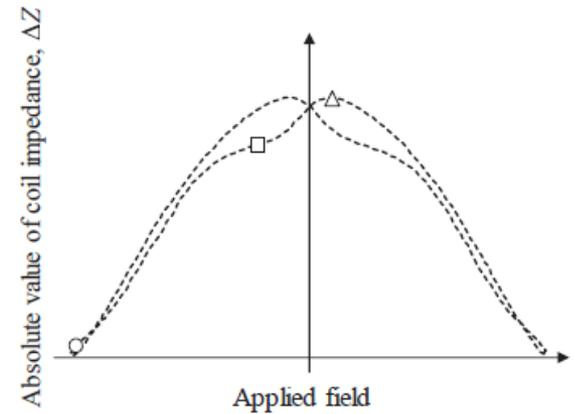
(a) Coil impedance as function of applied field
