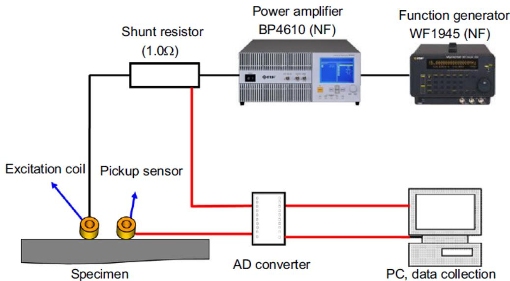
Fig. 6. Schematic of pulsed ECT experiment setup.
